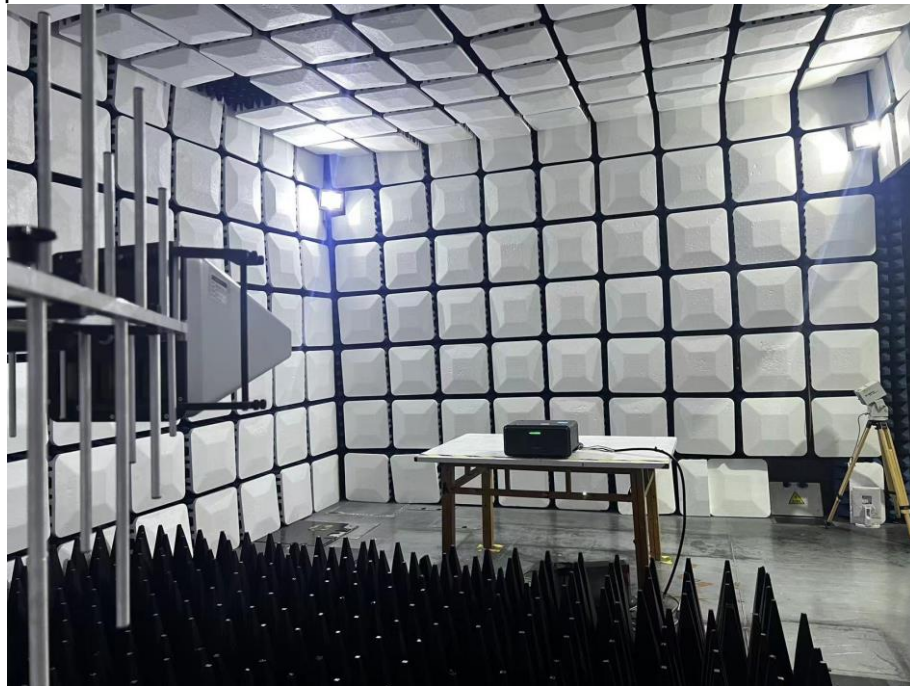
Photograph 2: Set-up for Radio-Frequency Electromagnetic Field (RS) Swept test & Spot test:
